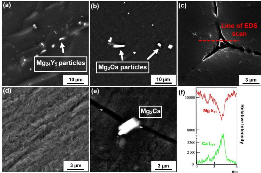
Fig. 4- FSEM micrographs of Mg-1Y (a,d) and Mg-1Ca (b,c,e) alloys in as-cast (a,b) and annealed (c,d,e) conditions, as well as the corresponding EDS line scan results of (c).
