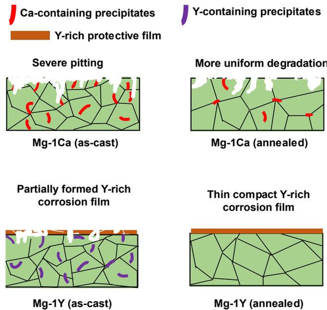
Fig. 7- Schematic illustration of the corrosion mechanism in Mg-1Ca and Mg-1Y alloys in as-cast and 96 h annealed conditions.
