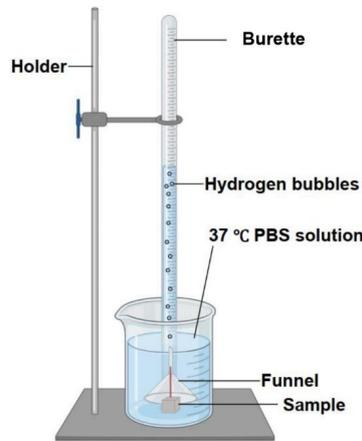
Fig. 1- Schematic illustration of the hydrogen evolution test [14].
