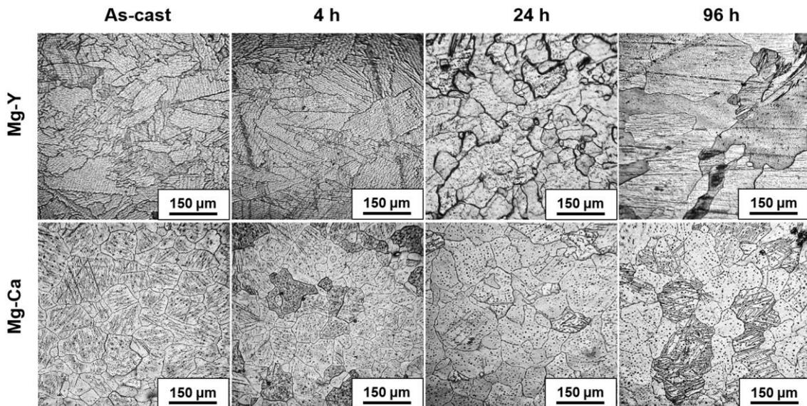
Fig. 2- Optical micrographs of the Mg–1Y and Mg–1Ca alloys in the as-cast and annealed (400 °C for 4, 24 and 96 h) conditions.
