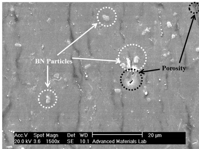
Fig. 3- Display the micro voids and agglomerated BN particles in SEM Microstructure of Al-4 wt.% BN is fabricated using mixing and hot extrusion.
