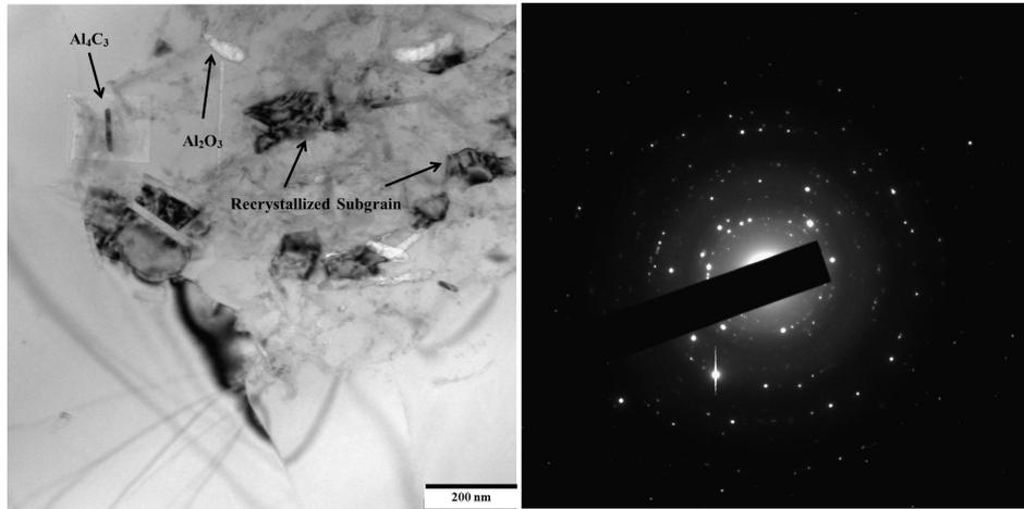
Fig. 4- TEM micrograph corresponding SAD pattern of Al-1 wt. % BN papered using planetary ball milling and hot extrusion.
