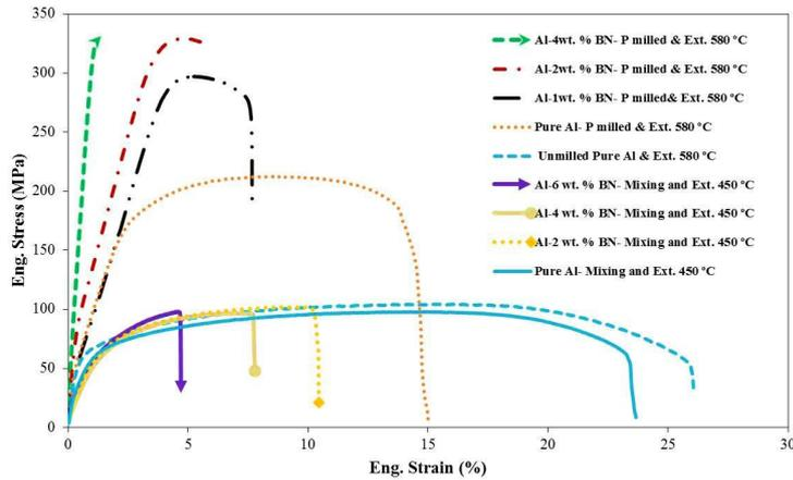
Fig. 2- Engineering Stress-strain curves for hot extruded samples including two powders preparation methods of ultrasonic mixing and planetary ball milling.
