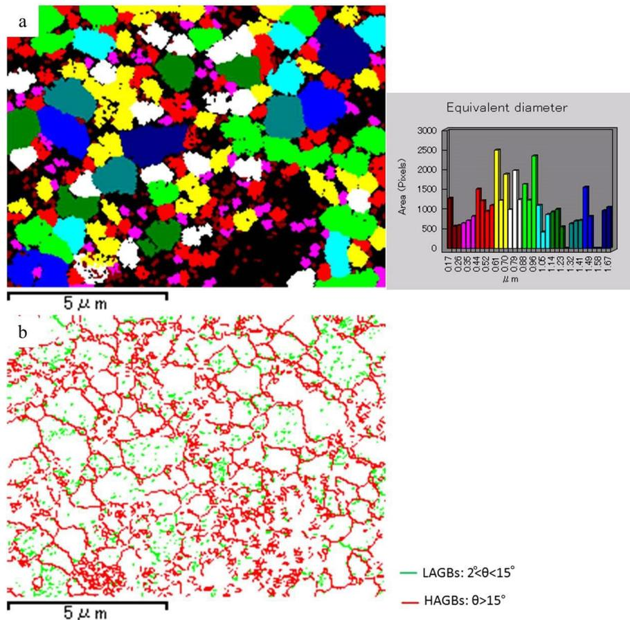
Fig. 6- a) EBSD map of Al-1 wt. % BN corresponding grain diameter distribution histogram b) grain boundary mapping.
