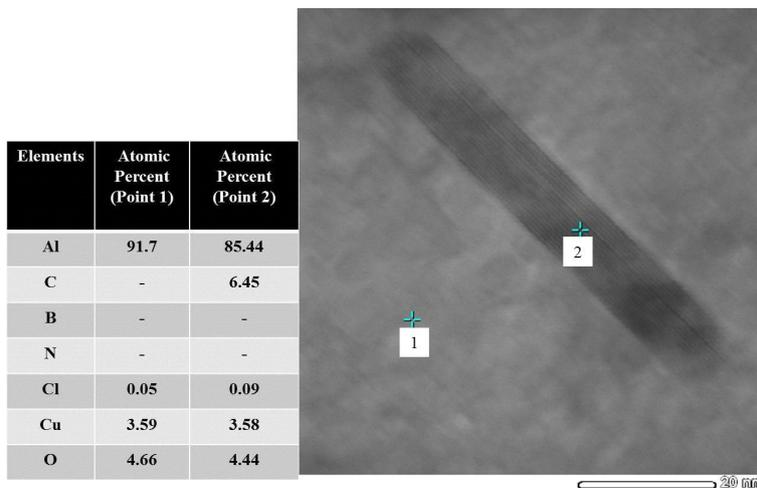
Fig. 5- Bright field corresponding of EDS results from in-situ  $Al_4C_3$  in Al-1 wt. % BN nanocomposite matrix.
