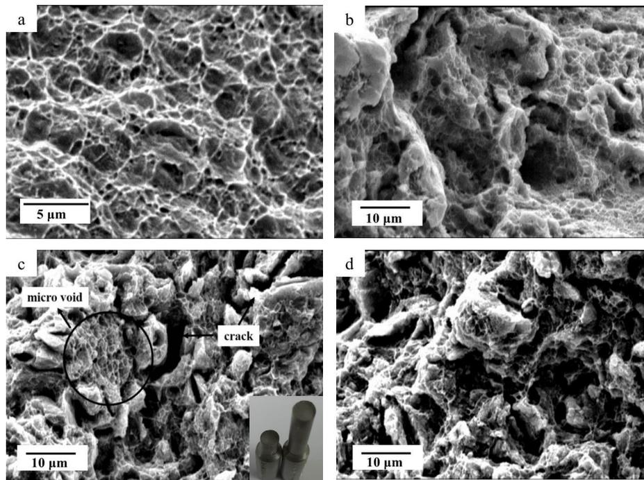
Fig. 7- Fracture surface of milled and extruded samples: a) pure Al b) Al-1 wt. % BN c) Al-2 wt. % BN d) Al-4 wt. % BN.
