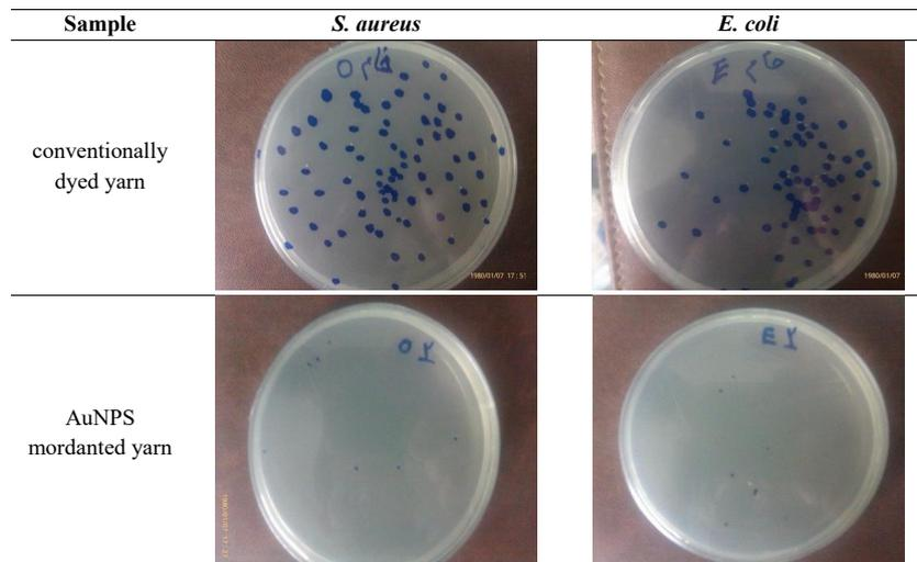
Fig. 5- Antibacterial properties of conventionally dyed woolen yarns and AuNPs mordanted one against *Staphylococcus aureus* and *Escherichia coli*.
