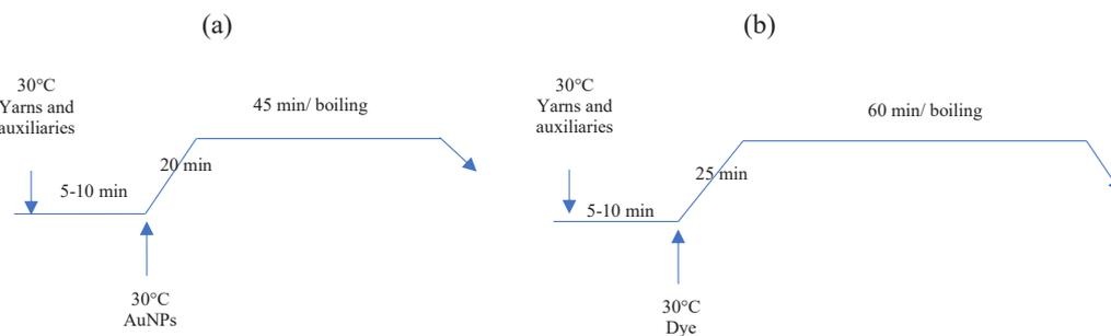
Fig. 1- The graph of (a) mordanting and (b) dyeing process.
