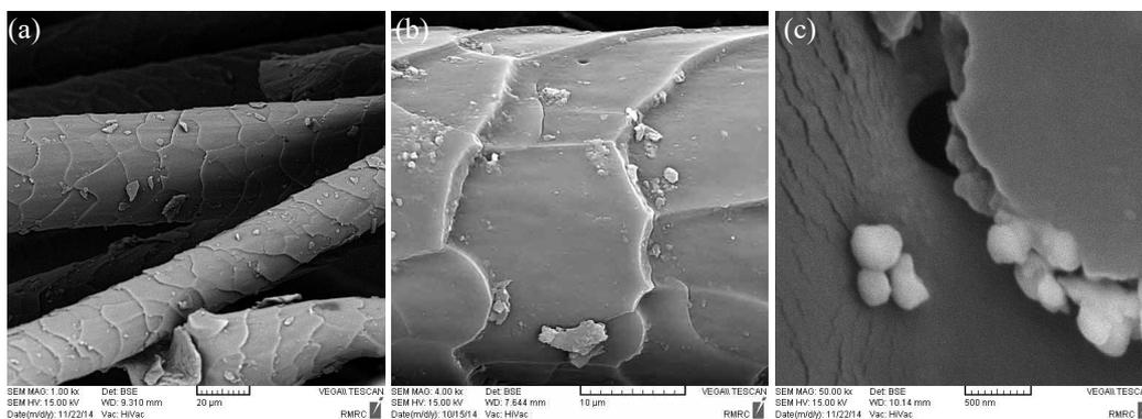
Fig. 4- SEM images of mordanted wool: a) yarn surface, b) fiber surface, and c) under the scale of wool fiber.
