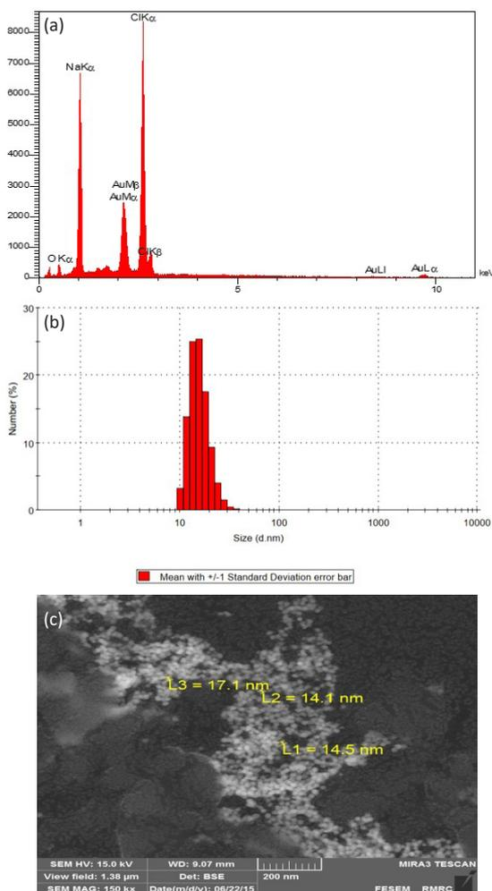
Fig. 3- (a) DLS, (b,) EDS, and (c) FESEM image of gold nanoparticles.
