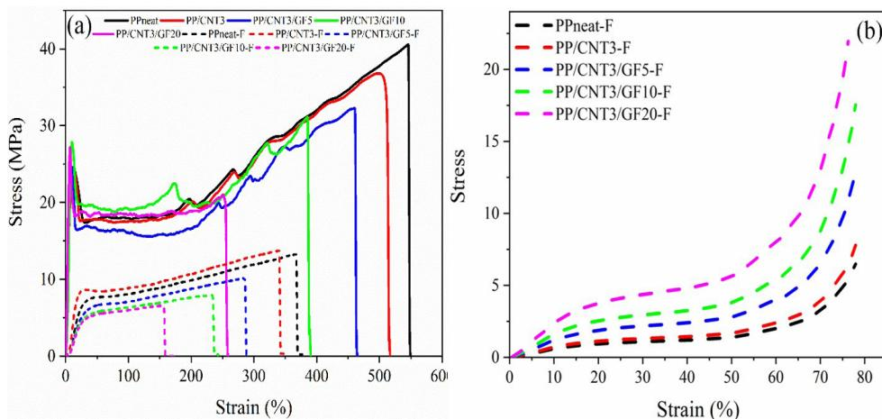
Fig. 4- Stress-strain curves of the samples in (a) tensile and (b) compression mode.
