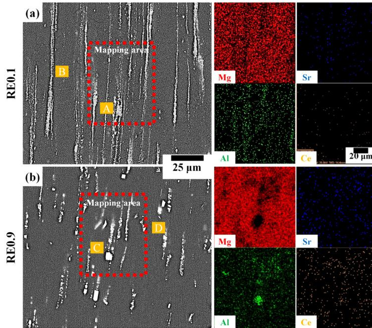
Fig. 2- SEM micrographs with the EDS analysis of the extruded RE0.1 and RE0.9 alloys.
