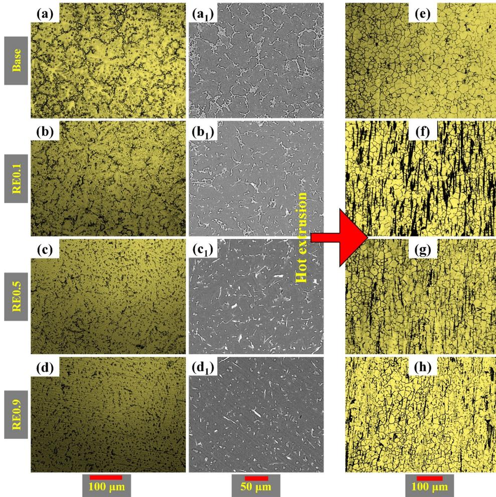
Fig. 1- Optical and SEM micrographs of the Mg-9Al-1Zn-RE/Sr alloys.
