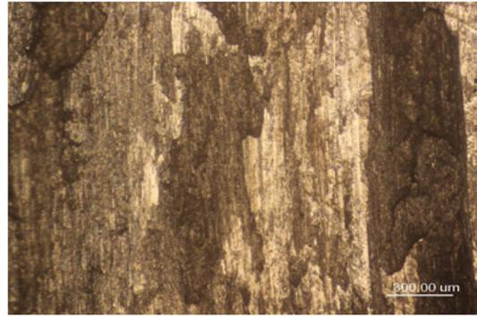
Fig. 13- The image of surface of the steel disc for nanostructured Aluminum at 200 °C.
