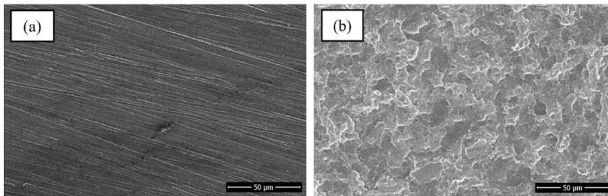
Fig. 1- SEM images of the surface of as received Mg (a) and after anodizing for 10 min (b).
