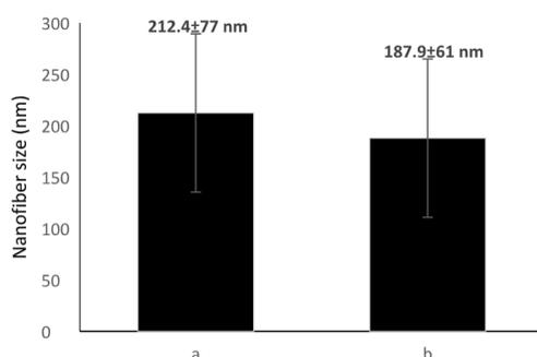
Fig. 7- Average diameter size of chitosan nanofibers (a) before addition of CNTs and (b) after addition of CNTs.
