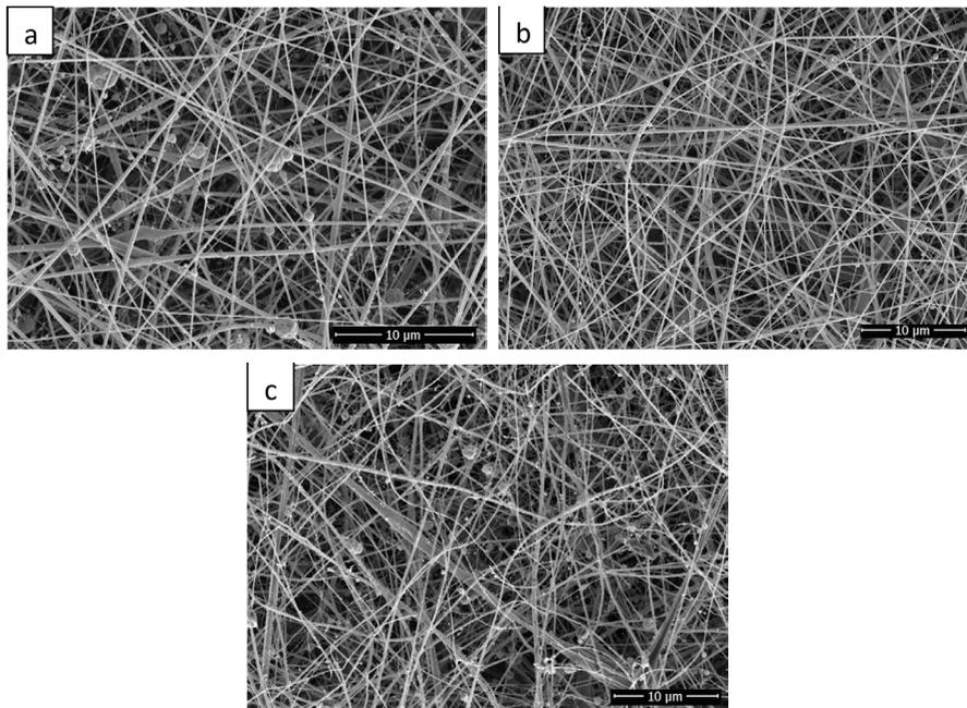
Fig. 2- FESEM images of composite nanofiber coatings achieved at feed rates of (a) 0.2, (b) 0.5 and (c) 0.8 ml / h (at 7% w/v chitosan concentration, 1% CNT with respect to chitosan concentration, distance=15 cm and voltage=20 kV).
