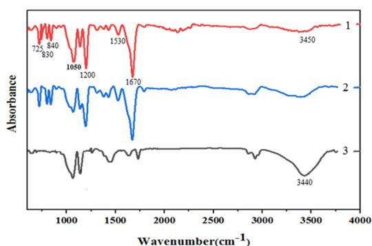
Fig. 9- FTIR spectra of nanofibers: (1) chitosan nanofibers, (2) nanocomposite fibers and (3) chitosan nanofibers after stabilization.
