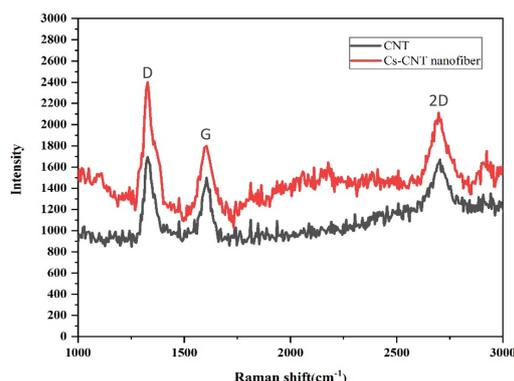
Fig. 10- Raman spectra: a) CNT and Chitosan-CNT composite coating.
