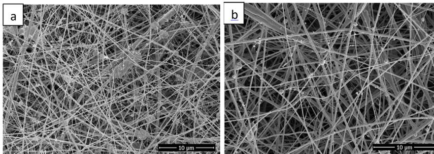
Fig. 3- FESEM images of composite nanofiber coatings achieved at voltage of (a) 15 and (b) 25 kV (at 7% w/v chitosan concentration, 1% CNT compare to chitosan concentration, distance=15 cm and feed rate= 0.5 ml / h).
