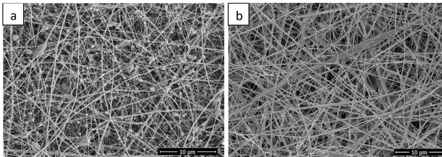
Fig. 4- FESEM images of composite nanofibers fabricated at tip to collector distance of (a) 10 and (b) 20 cm (at 7% w/v chitosan concentration, 1% CNT compare to chitosan concentration, 20 kV and 0.5 ml / h feed rate).
