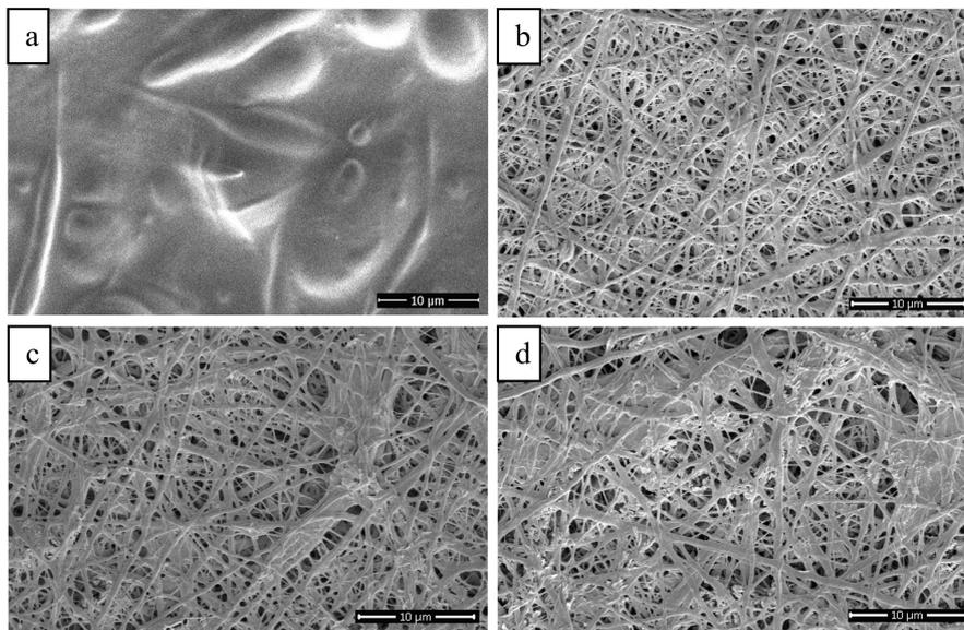
Fig. 8- FESEM images of non-stabilized specimen after contact with water (a) and stabilized specimens in sodium carbonate solution for (b) 10, (c) 25 and (d) 40 min. (Electrospinning time was 75 min).
