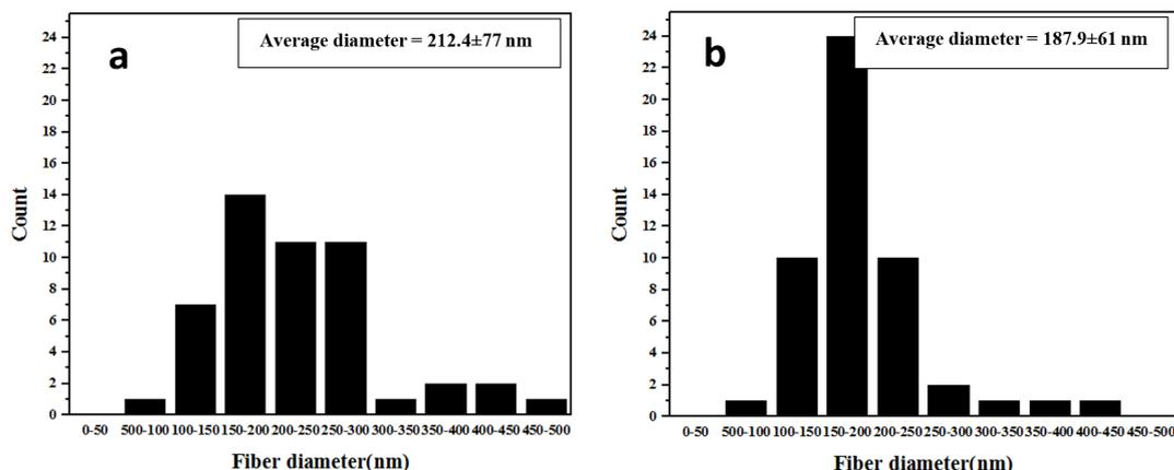
Fig. 6- Average and size distribution of nanofiber coatings; a) Chitosan fibers and b) composite fibers.
