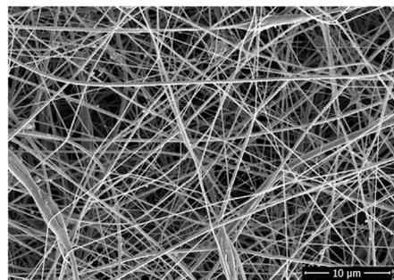
Fig. 5- FESEM images of chitosan nanofiber coating achieved at 7% w/v chitosan concentration, 1% CNT compare to chitosan concentration, 20 kV, 15 cm distance and 0.5 ml / h feed rate.
