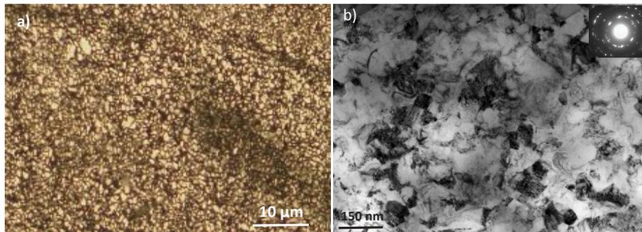
Fig. 1- a) Microstructure of the experimental alloy ECAP processed at 200 °C, b) TEM of recrystallized grain structure.
