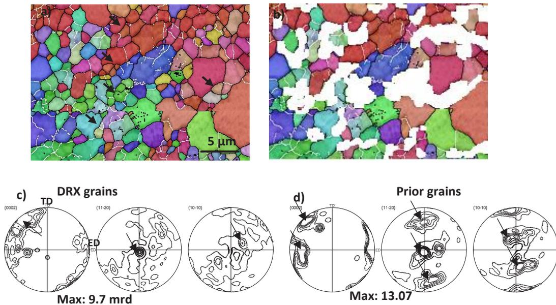
Fig. 3- (a) EBSD image showing the microstructure of AZ31 alloy ECAPed up to one pass, EBSD map with b) excluded parent grains, c) pole figures of DRX grains, d) pole figures of parent grains.
