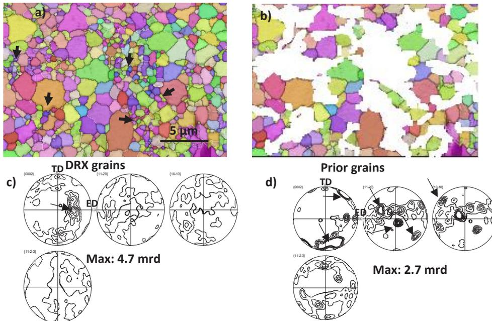
Fig. 4- (a) EBSD image showing the microstructure of AZ31 alloy ECAPed up to two passes, EBSD map with b) excluded parent grains, c) pole figures of DRX grains, d) pole figures of parent grains.
