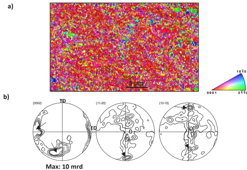
Fig. 2- a) IPF, b) PFs of the experimental alloy deformed up to four ECAP passes.
