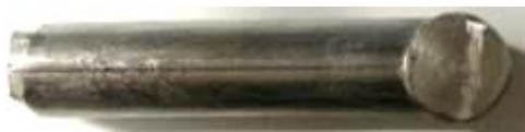
Fig. 3- Shape of the sample after 14 passes ECAP in the die with choked exit channel.
