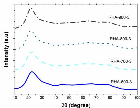
Fig. 1- XRD patterns of samples calcined at various temperatures.
