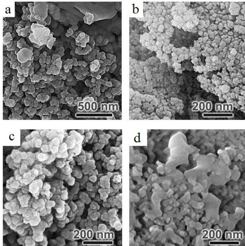
Fig. 2- FE-SEM images of processed samples: RHA-600-3(a), RHA-700-3(b), RHA-800-2(c), and RHA-900-8 (d).
