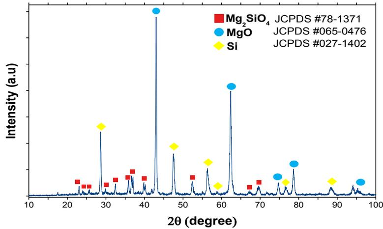
Fig. 3- X-ray powder diffraction pattern of synthesized composite.
