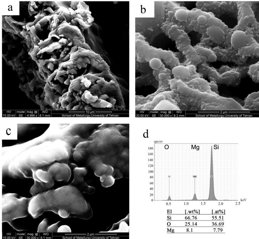
Fig. 4- HRSEM images of Si-MgO- $Mg_2SiO_4$  particles prepared by magnesiothermic reduction process (a, b,c) and corresponding EDS spectrum (d).
