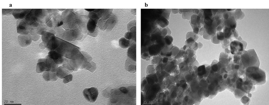
Fig. 3- TEM images of CuO nanoparticles prepared from copper(II) iodide in the presence of catsc (a) and mecatsc (b).
