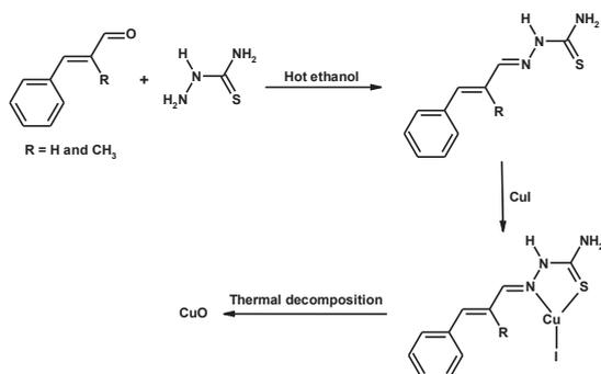
Scheme. 1- Schematic illustration of the formation of CuO nanoparticles.
