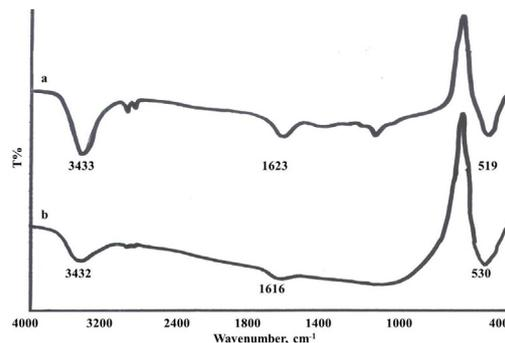
Fig. 1- The FT-IR spectra of CuO nanoparticles prepared from copper(I) iodide in the presence of catsc (a) and mecatsc (b).
