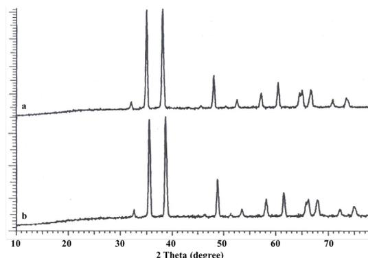
Fig. 2- XRD patterns of CuO nanoparticles prepared from copper(I) iodide in the presence of catsc (a) and mecatsc (b).
