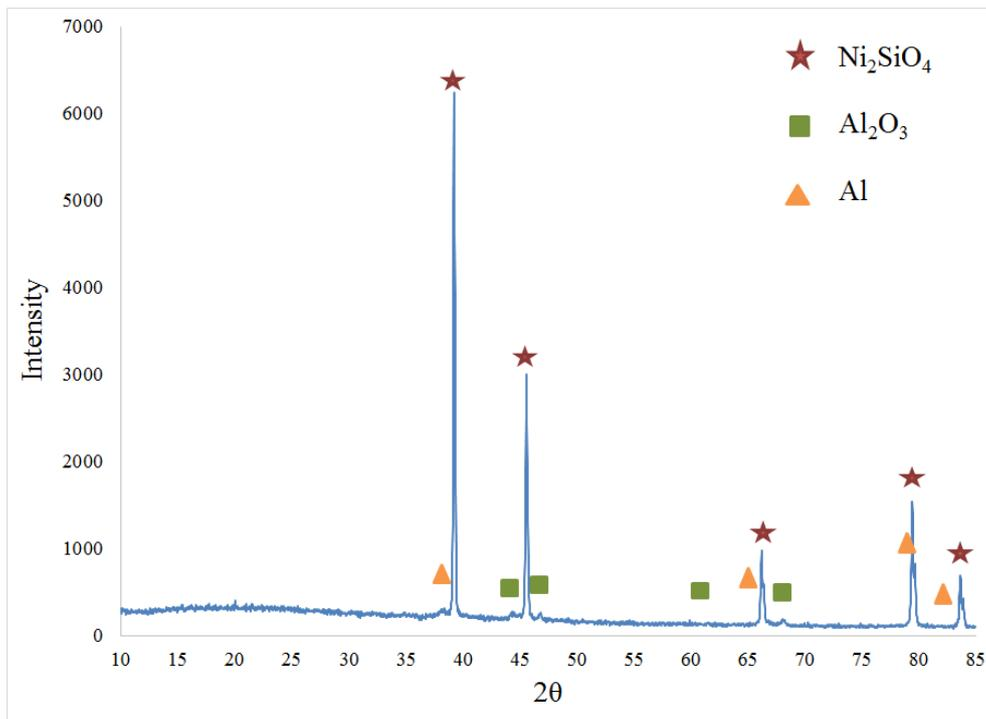
Fig. 7. Pattern of GIXRD on the A-25-40 sample
