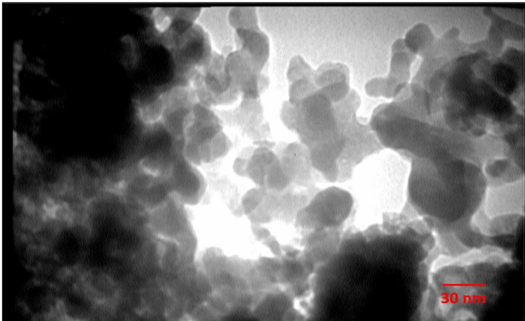
Fig. 1. TEM picture of  $\text{Si}_3\text{N}_4$  nano-powder
