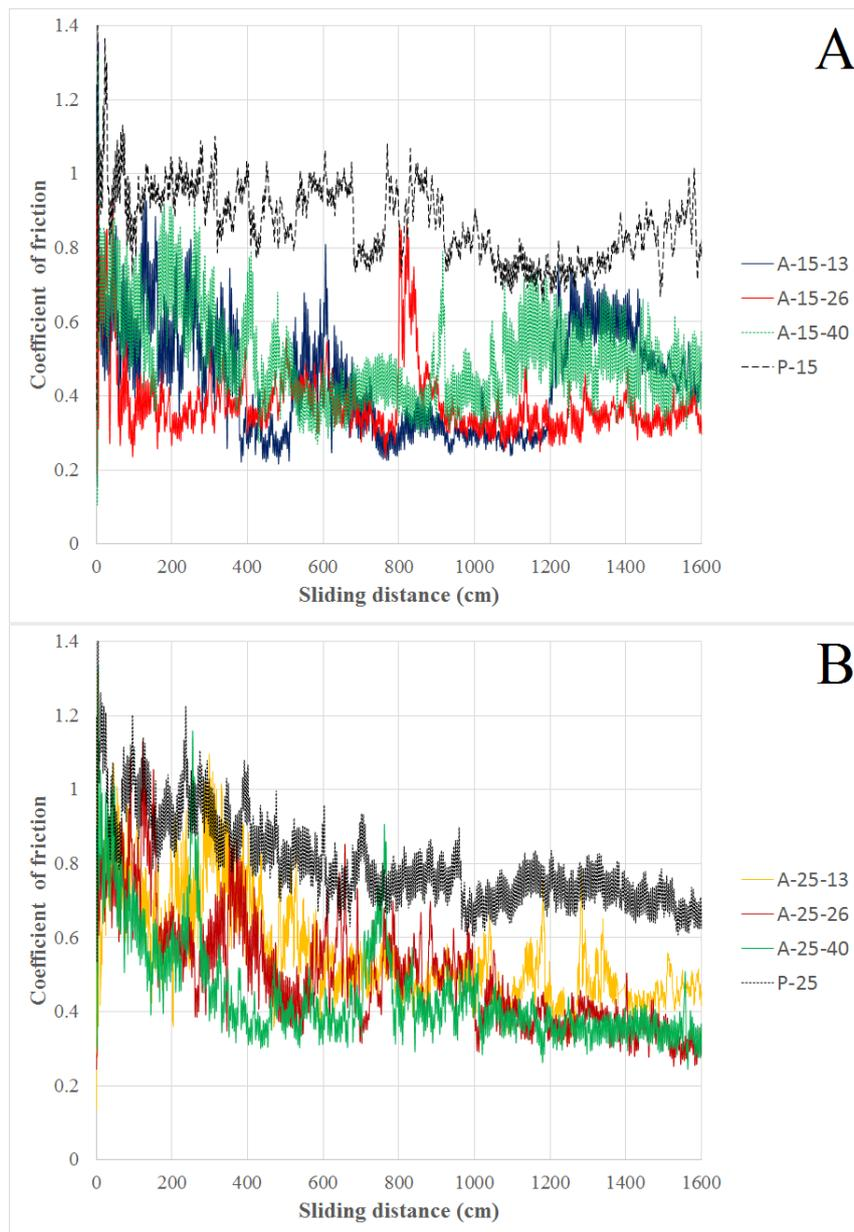
Fig. 11. Coefficient of friction changes curve based on eroded distance for samples coated with current density of (A) 15 mA/cm<sup>2</sup> (B) 25 mA/cm<sup>2</sup>
