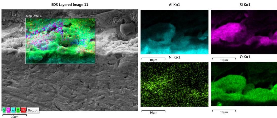
Fig. 5. SEM image of cross section related to A-25-40 sample with elemental analysis map
