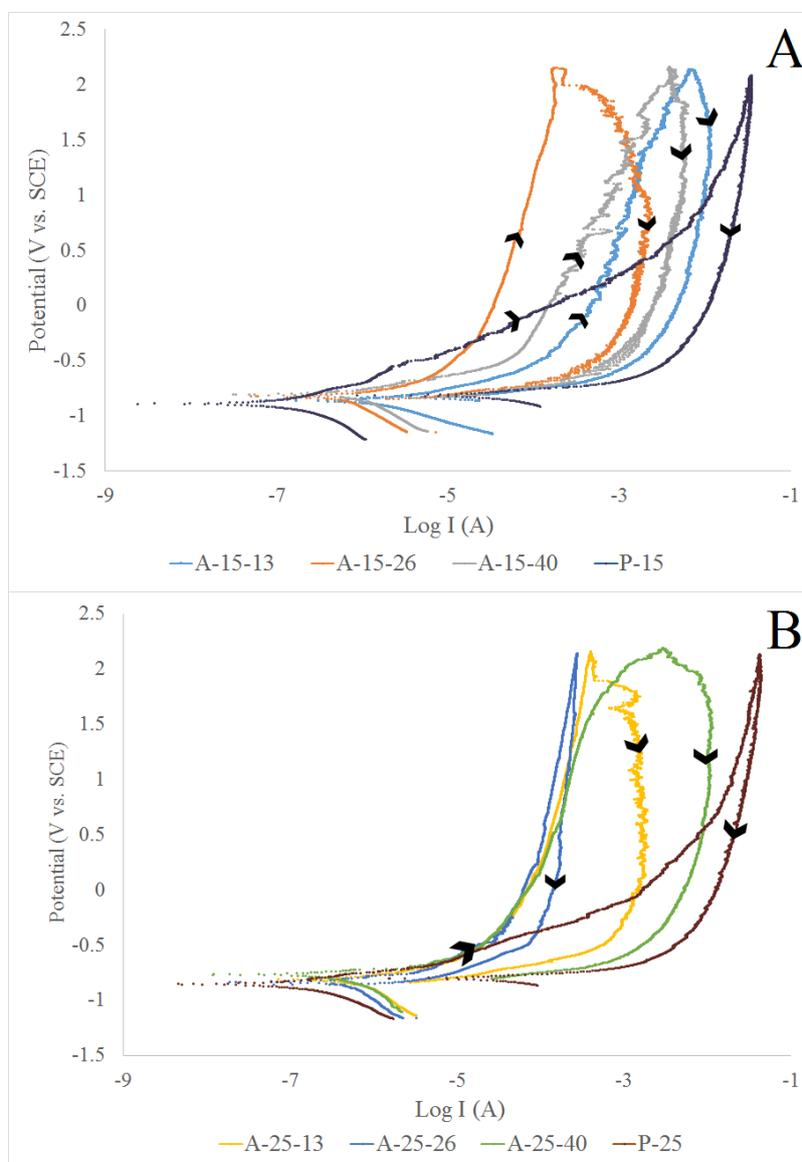
Fig. 10. Cyclic Potentiodynamic polarization curves of different treated samples after 24 hours of immersion in 3.5% NaCl solution
