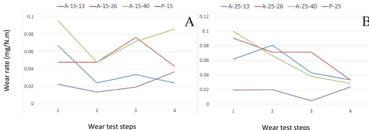
Fig. 12. Wear rate at each step of wear testing for (A) 15 mA/cm<sup>2</sup> (B) 25 mA/cm<sup>2</sup> samples
