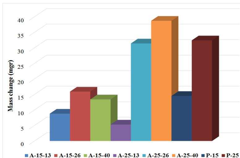
Fig. 9. Graph of the weight changes in samples before and after the coating
