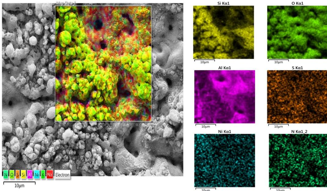
Fig. 4. SEM image of coating surface related to A-25-40 sample with elemental analysis map
