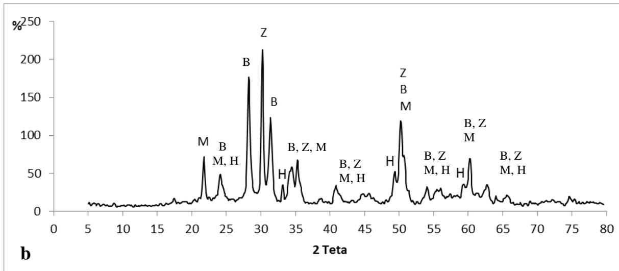
Fig. 4. XRD pattern of sample a) raw sample 5M and b) annealed sample 5M. M: muscovite H: hematite (PDF 33-0664), B: baddeleyite (PDF 72-1669) and Z: zirconium oxide (PDF 79-1771)
