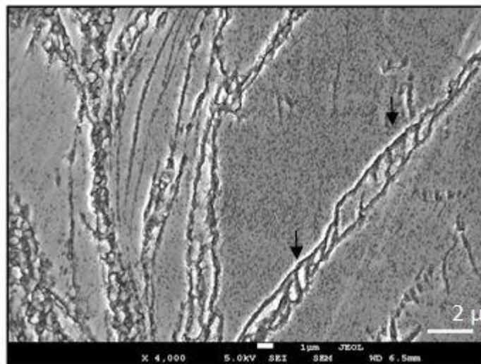
Fig. 6. Recrystallized grains within twin during in an ABE AZ31 alloy
