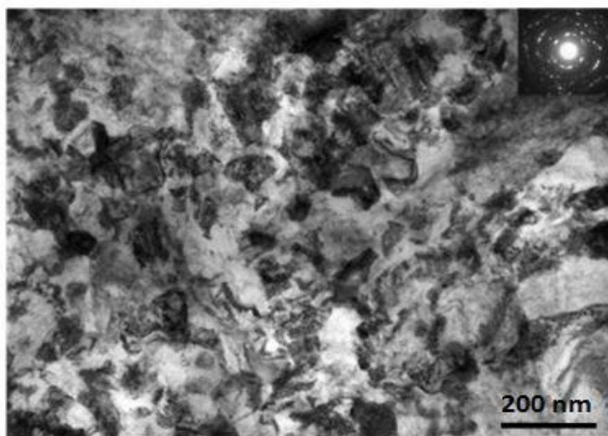
Fig. 1. Typical nano grains developed after single pass ABE
