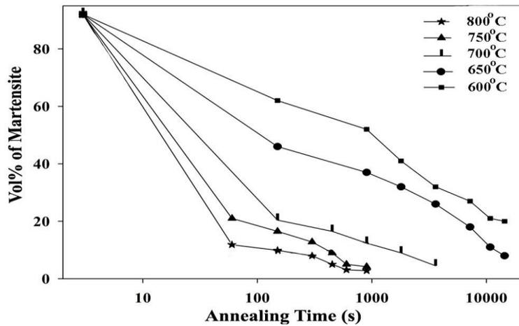
Fig. 5. Vol% of Martensite vs. annealing time at various reversion temperatures as determined by magnetic measurements
