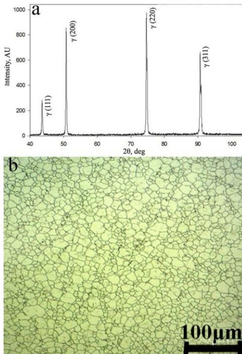
Fig. 2. a) X-ray diffraction pattern of the as-received material, b) the corresponding optical micrograph
