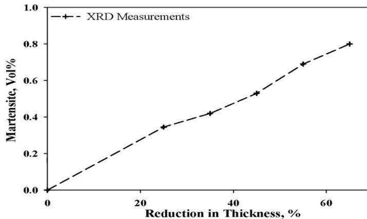
Fig. 3. Volume fraction of  $\alpha'$ -martensite as a function of cold reduction in AISI 304L ASS at  $25^\circ\text{C}$
