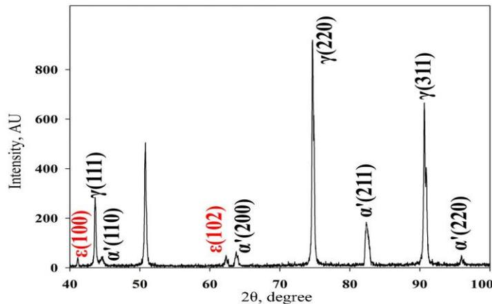
Fig. 4. X-ray diffraction pattern of the cold rolled ( $10^\circ\text{C}$ ) AISI 304L stainless steel
