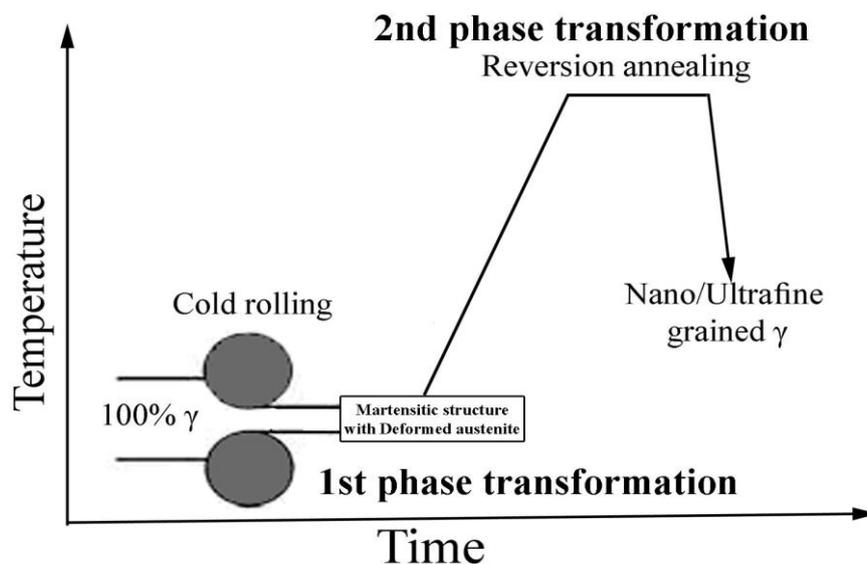
Fig. 1. Schematic of advanced thermomechanical process used to obtain Nano/ ultrafine grained austenitic stainless steel [4]
