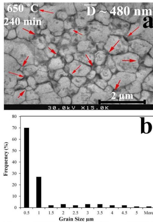
Fig. 6. SEM image taken from the microstructure of sample annealed at 650°C for 240 min, and the corresponding grain size histogram
