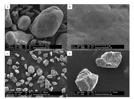
Fig. 1- Morphology of Al-2 wt. % BN composite powders after two different preparation methods a, b) Ultrasonic Mixing method with high magnification view on Al particle with uniform distribution of BN particles c, d) 300 min planetary ball milling process with high magnification view.
