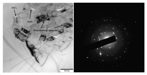
Fig. 4- TEM micrograph corresponding SAD pattern of Al-1 wt. % BN papered using planetary ball milling and hot extrusion.
