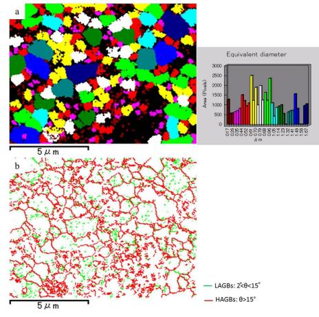
Fig. 6- a) EBSD map of Al-1 wt. % BN corresponding grain diameter distribution histogram b) gain boundary mapping.
