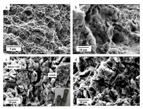
Fig. 7- Fracture surface of milled and extruded samples: a) pure Al b) Al-1 wt. % BN c) Al-2 wt. % BN d) Al-4 wt. % BN.
