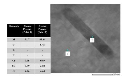
Fig. 5- Bright field corresponding of EDS results from in-situ Al<sub>4</sub>C<sub>2</sub> in Al-1 wt. % BN nanocomposite matrix.
