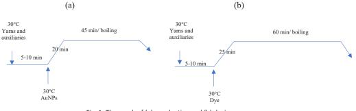
Fig. 1- The graph of (a) mordanting and (b) dyeing process.
