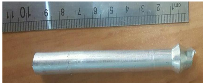
Fig. 2- Aluminum sample during HCEE without back pressure from the unprocessed zone to the processed zone.
