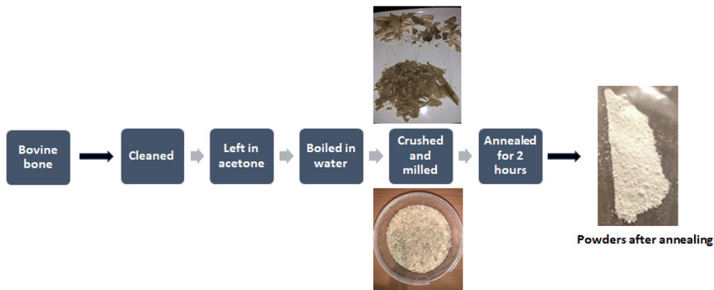
Fig. 1- Schematic of the processing stages starting from as-received bone to hydroxyapatite powder.
