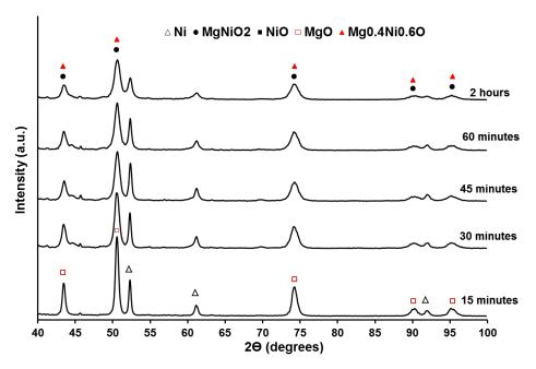
Fig. 1- XRD patterns of the Mg-NiO system as a function of milling time (the as-milled samples).
