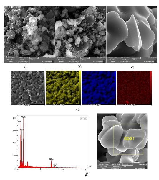
Fig. 4- SEM micrographs of the 30 minutes milled mixture after one hour heating at different conditions. (a) 400 OC in argon atmosphere, (b) 400 OC in ambient air, (c) 1000 OC in argon atmosphere, (d) elemental map analysis of the heated sample at 1000 OC in argon atmosphere, (e) EDS analysis of the heated sample at 1000 OC in argon atmosphere.
