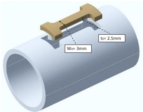
Fig. 2- Dimension of a tensile test specimen.
