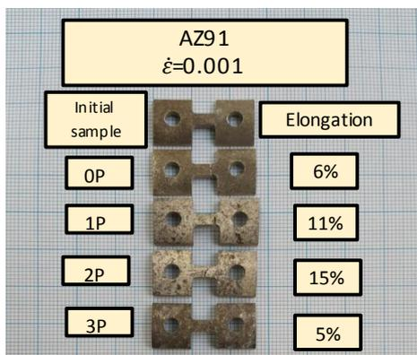
Fig. 5- Fractured specimens after the tensile test.
