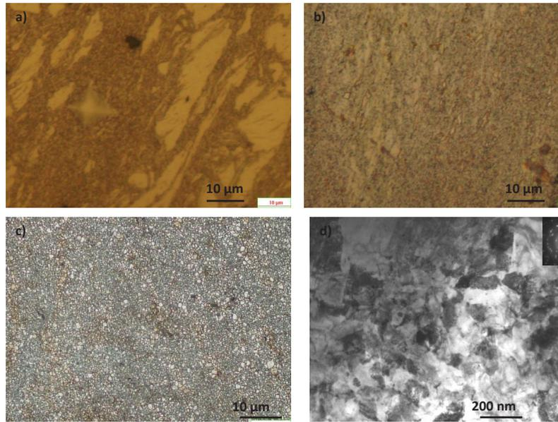
Fig. 3- Microstructure of the experimental alloy deformed up to a) one, b) two, c) four passes at 280 °C, d) ultrafine/nano grains formed after two-pass ABE processing.
