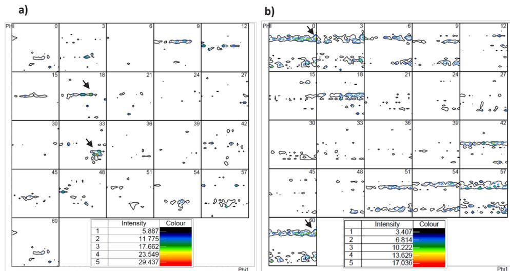
Fig. 8- ODF sections measured from the processed AZ31 alloy ABEed up to a) one pass, b) two passes.
