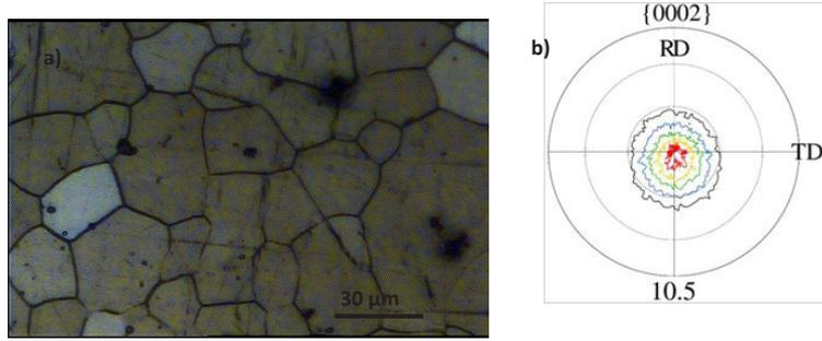
Fig. 1- a) Initial microstructure, b) measured basal pole figure of the experimental as-rolled AZ31 alloy.
