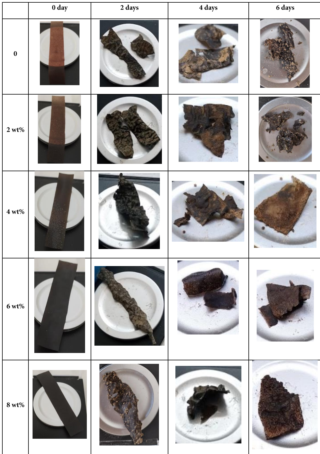
Fig. 7- Soil burial test of BP starch and BP-ECG biopolymers with different filler loading.
