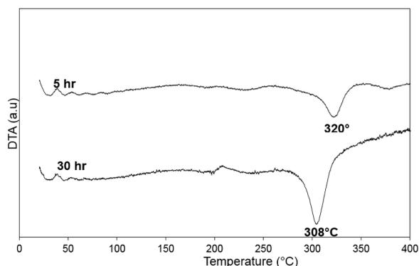
**Fig. 5.** DTA curves of MgH<sub>2</sub>-ZrB<sub>2</sub> composite at selected milling times.
