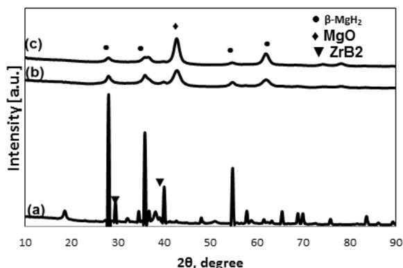
**Fig. 4.** X-ray diffraction patterns of MgH<sub>2</sub>-10 wt.% ZrB<sub>2</sub> composite at different milling times: (a) 0 h, (b) 5 h, (c) 30 h.
