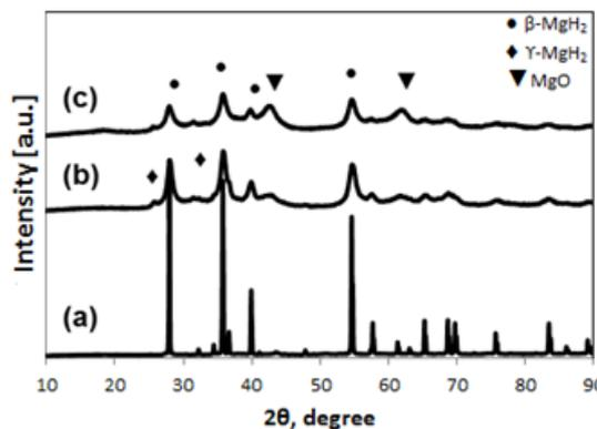
**Fig. 1.** X-ray diffraction patterns of pure  $\text{MgH}_2$  powder at different milling times: (a) 0 h, (b) 5 h, and (c) 30 h.
