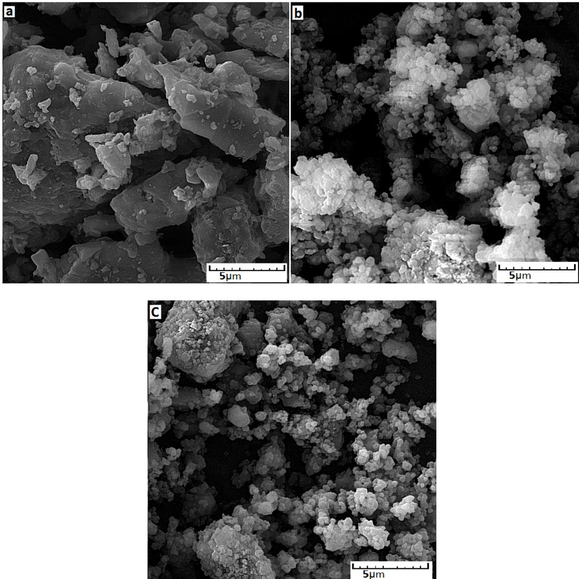
**Fig. 6.** SEM micrographs showing the morphology of  $\text{MgH}_2$ -10 wt%  $\text{ZrB}_2$  after mechanical alloying for: (a) 0 h, (b) 5 h, and (c) 30 h.
