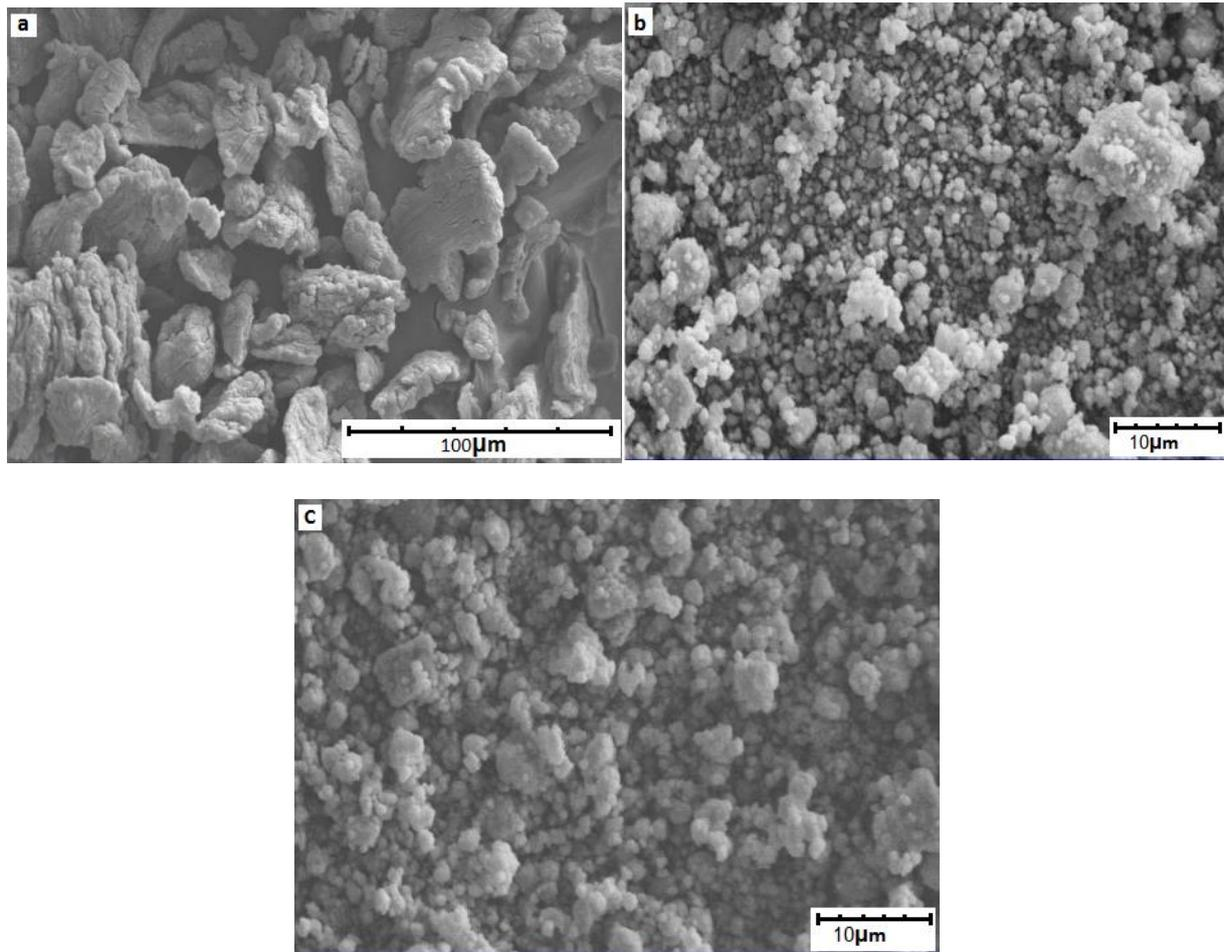
**Fig. 2.** SEM micrographs of magnesium hydride powder for un-milled (a) and milled for 5 h (b) and 30 h (c).
