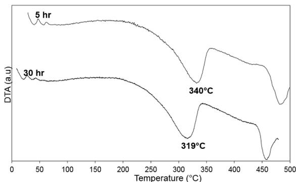
**Fig. 3.** DTA curves of pure  $\text{MgH}_2$  milled for different times.
