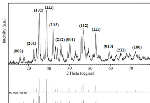
**Fig. 1.** XRD pattern of as synthesized Bi<sub>2</sub>S<sub>3</sub> nanorods at 50 W for 30 min (sample 3).
