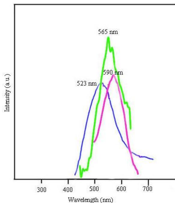
**Fig. 4.** PL spectrum of the as synthesized Bi<sub>2</sub>S<sub>3</sub> nanorods (a) sample 2 (b) sample 3 (c) sample 8.
