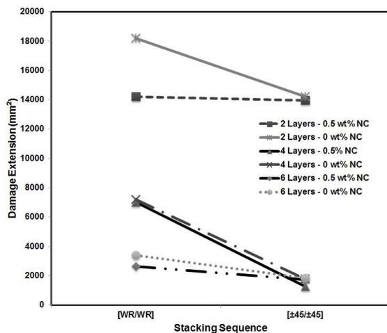
**Fig. 8.** Comparison of damage extension between with and without nanoclay (NC) samples under single hail ice impact.
