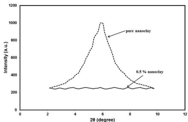
**Fig. 9.** XRD patterns of Epoxy-Cloisite30B nanocomposites and pure Cloisite30B.
