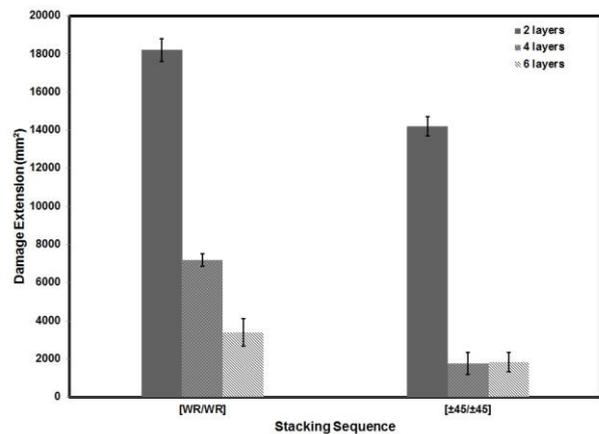
**Fig. 6.** Damage extension vs. different stacking sequence of two, four and six layered composite panels under hail ice impact.
