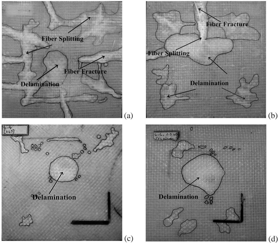
**Fig. 4.** Damage extension for (a) Sample [WR/WR] two layered, (b) Sample [WR/WR] two layered with nanoclay, (c) Sample  $[\pm 45^\circ/\pm 45^\circ]_s$  four layered, (d) Sample  $[\pm 45^\circ/\pm 45^\circ]_s$  four layered with nanoclay.
