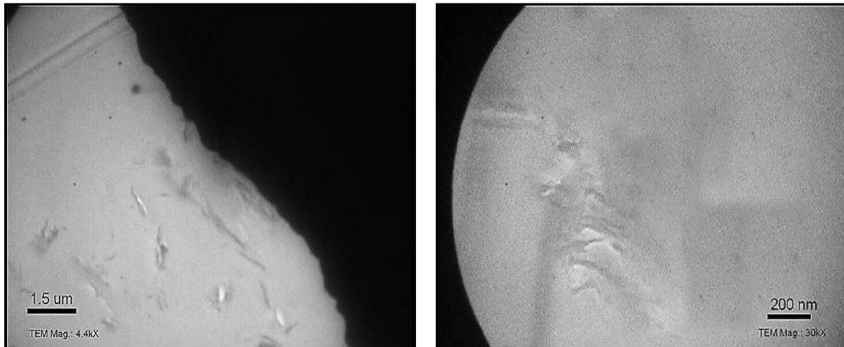
**Fig. 10.** TEM micrograph of specimen containing 0.5 wt.% nanoclay.
