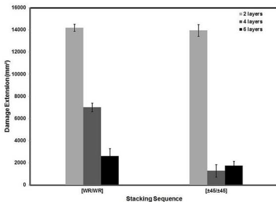
**Fig. 7.** Damage extension vs. different stacking sequence of two, four and six layered nanocomposite panels under hail ice impact.
