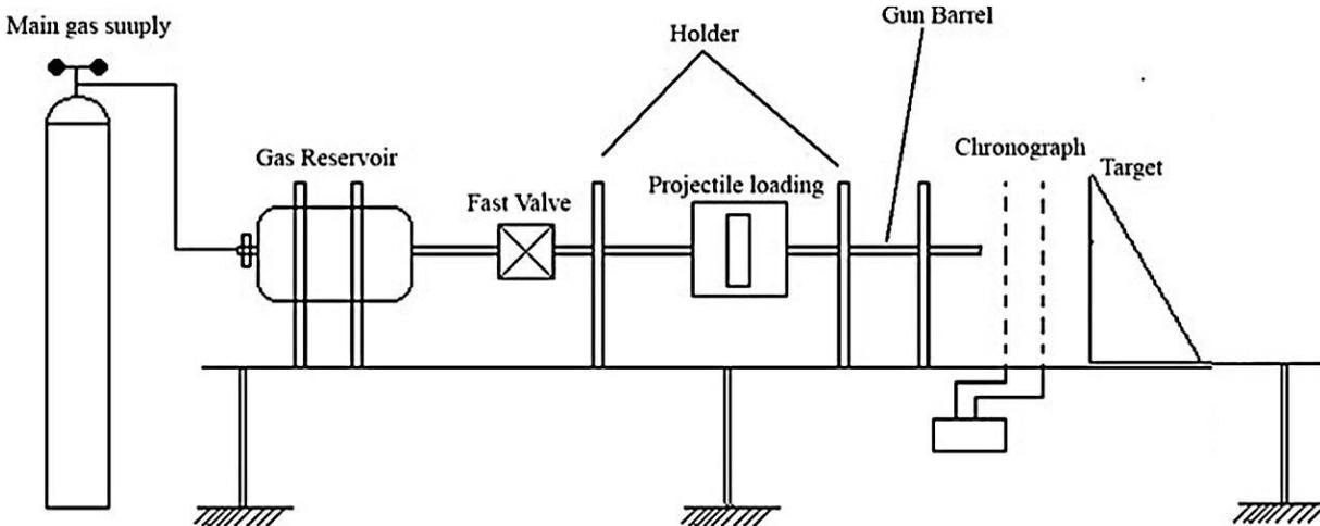
**Fig. 1.** Schematic representation of high velocity impact testing device (gas gun).
