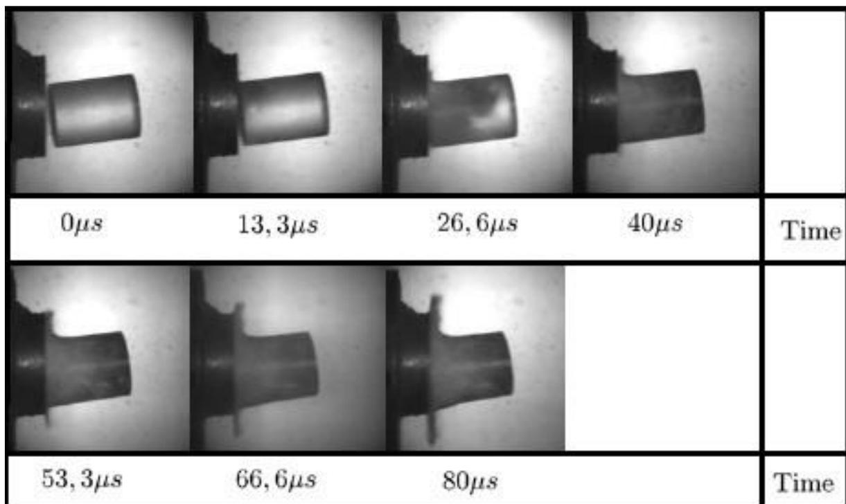
Fig. 3. The failure history for a cylindrical ice [22]
