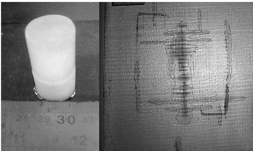
**Fig. 2.** (a) Moulded ice projectile. (b) Dark area showing damage extension area after impact.
