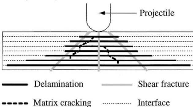
**Fig. 5.** Illustration of impact damage in a laminate. [23]
