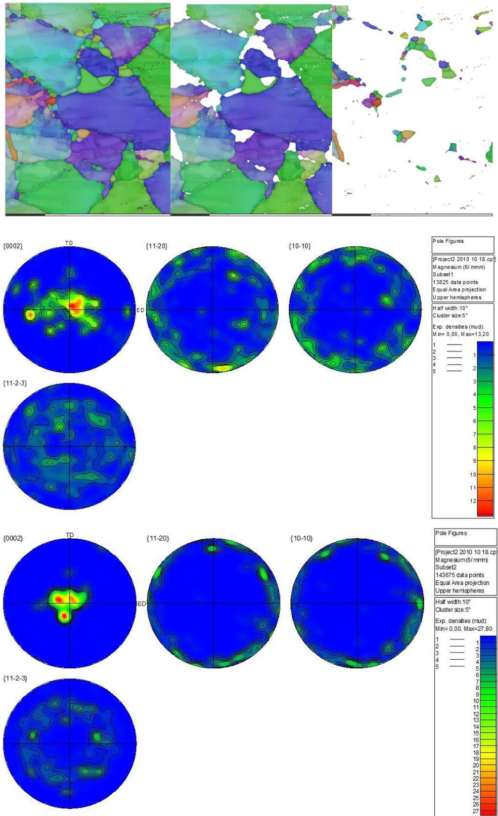
**Fig. 3.** (a) EBSD image showing the microstructure of AZ31 alloy ABEed at 330 °C, EBSD map with b) excluded parent grains, c) excluded recrystallized grains, d) pole figures of DRX grains, e) pole figures of parent grains.
