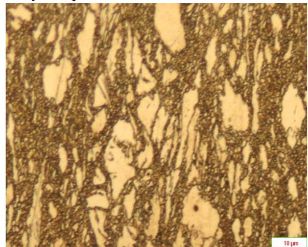
**Fig. 1.** Optical microstructure showing bimodal grain distribution obtained after middle stage of ABE.
