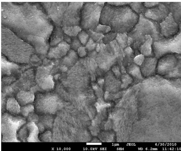
**Fig. 2.** SEM micrograph showing recrystallized grain along prior grain boundaries during ABE.
