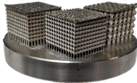
Fig. 2- Example of parts produced by SLM technique fastened to the build plate with supports [22].
