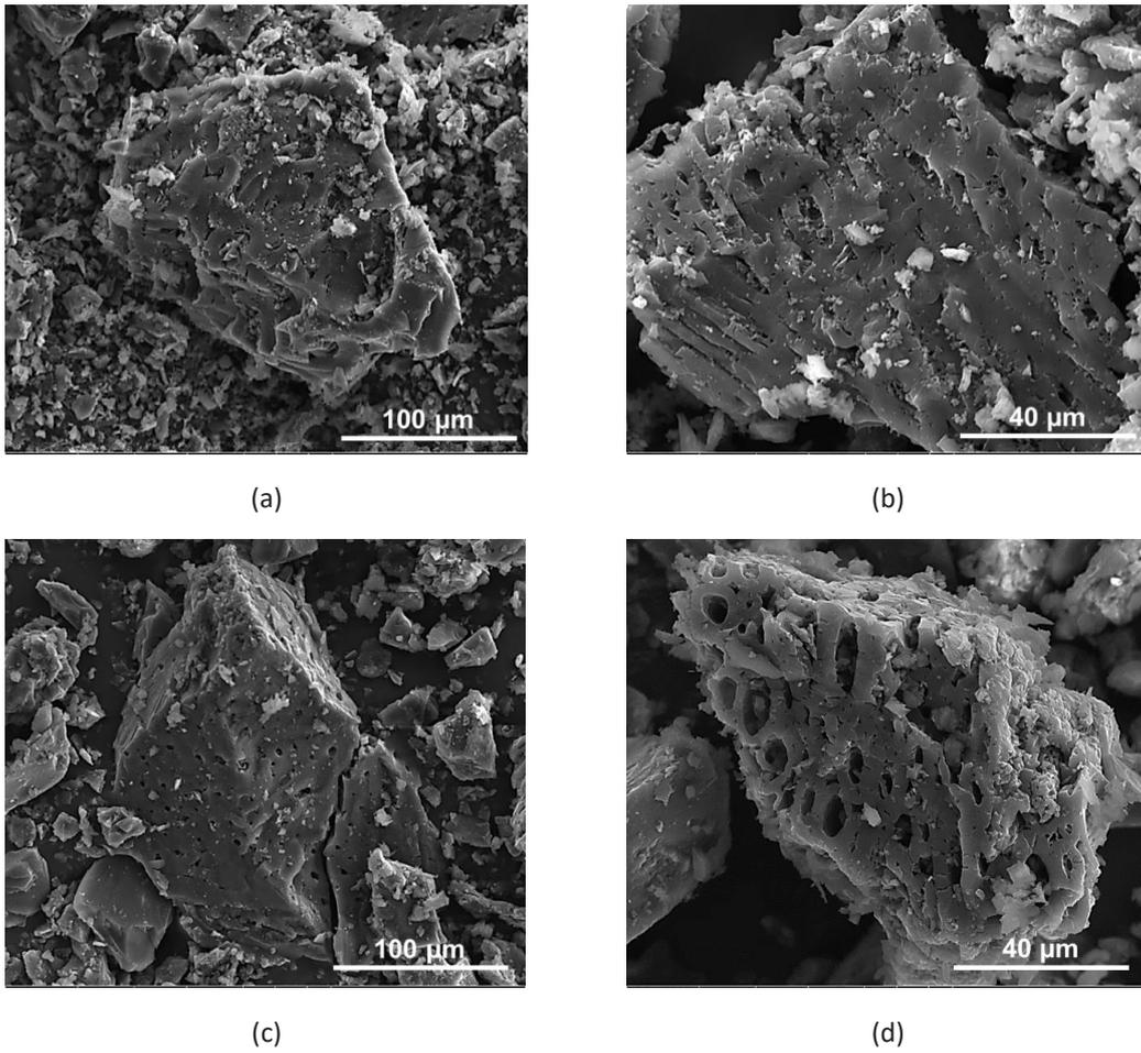
Fig. 1- Scanning Electron Microscope (SEM) of the coconut-waste biochar pyrolyzed at (a, b) 400 °C and (c, d) 500 °C. The (a) and (b) were captured at a low magnification. The (c) and (d) were captured at a high magnification.
