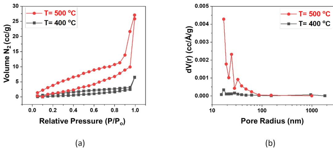
Fig. 2- (a) Nitrogen desorption/adsorption isotherms and (b) Pore size distribution of the coconut-waste biochar pyrolyzed at 400 °C (black line-symbol) and 500 °C (red line-symbol).
